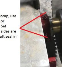
If installing a comp, use either the top or bottom ports. Set screws on the sides are to hold the shaft seal in place.
