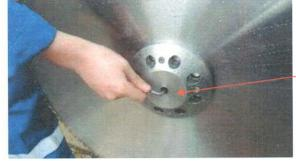
2. Slacken and remove the centre hub retaining bolt
