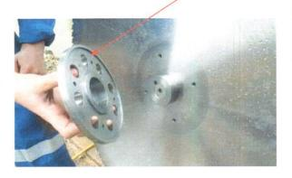
4. Fit new blade, ensuring the correct number of shims are placed between end of motor shaft and front hub for a gap between rear of hub and ram bolt. Generally this will be 4 shims to create a space of 4-5mm
