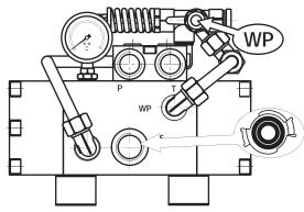
HPW-PUMP EQUIPPED WITH WATER PRESSURE UNLOADER VALVE
