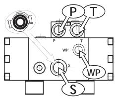
HPW-PUMP WITHOUT WATER PRESSURE UNLOADER VALVE
