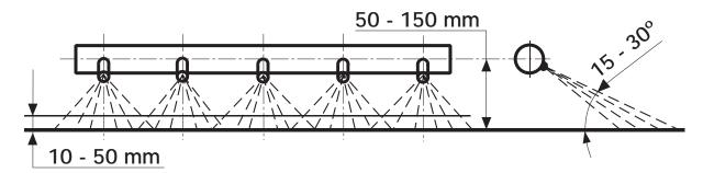
When adjusting on-position, the street washing pipe should be brought down horizontally as close as possible to the roadway. An operator should be careful, though most KPL-types are provided with support wheel in order to prevent street washing pipe from damage. Street washing pipe should be positioned in relation to surface to be washed so, that each water jet would meet its adjoiners at a distance of 10—50 mm from it (refer to the drawing above).
