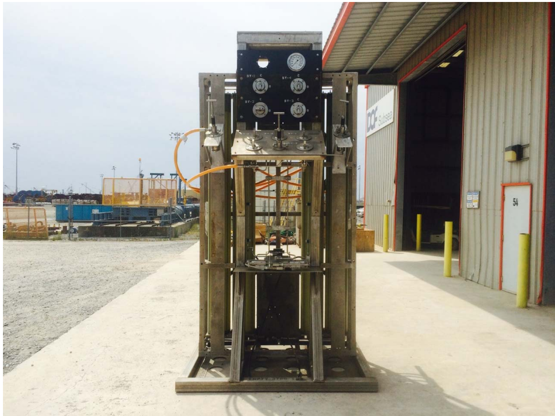
Figure 3.1-1: Hydrate Remediation Skid (Front)
