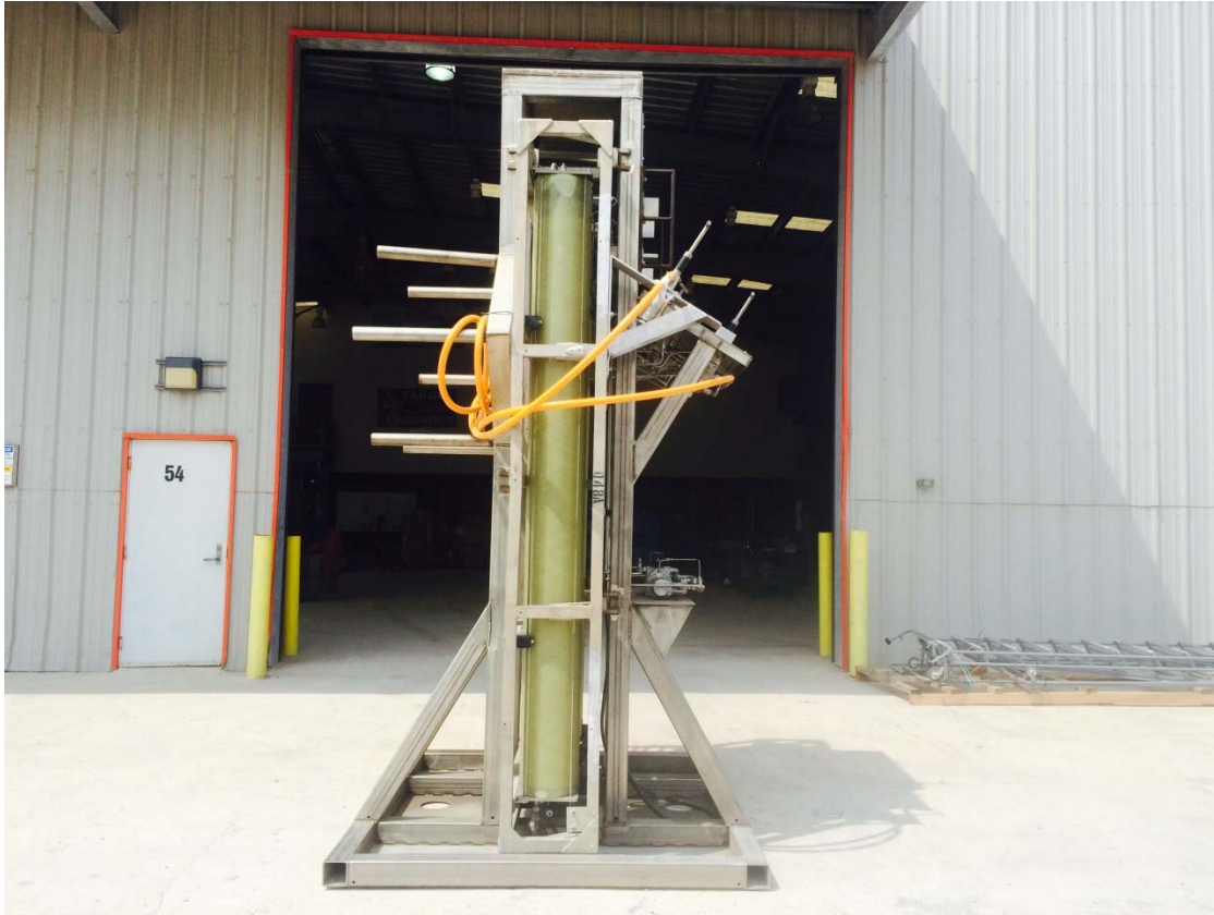
Figure 3.1-2: Hydrate Remediation Skid (Side)
