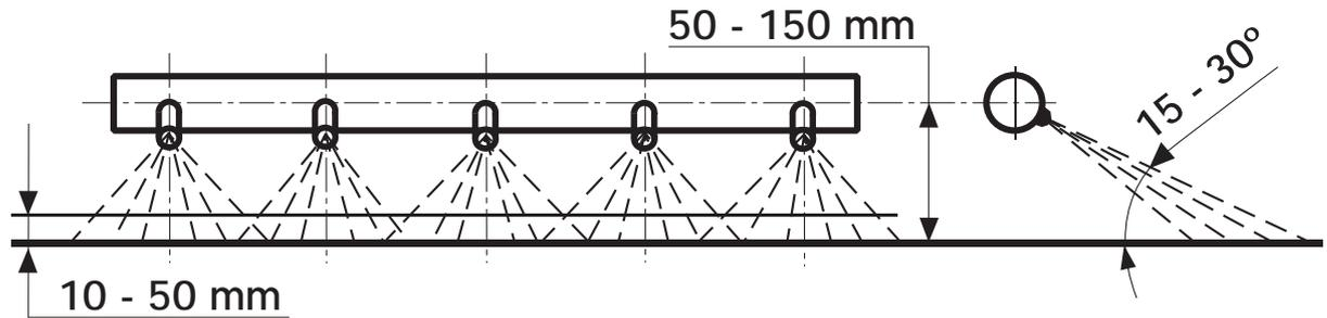
When adjusting on-position, the street washing pipe should be brought down horizontally as close as possible to the roadway. An operator should be careful, though most KPL-types are provided with support wheel in order to prevent street washing pipe from damage. Street washing pipe should be positioned in relation to surface to be washed so, that each water jet would meet its adjoiners at a distance of 10–50 mm from it (refer to the drawing above).
