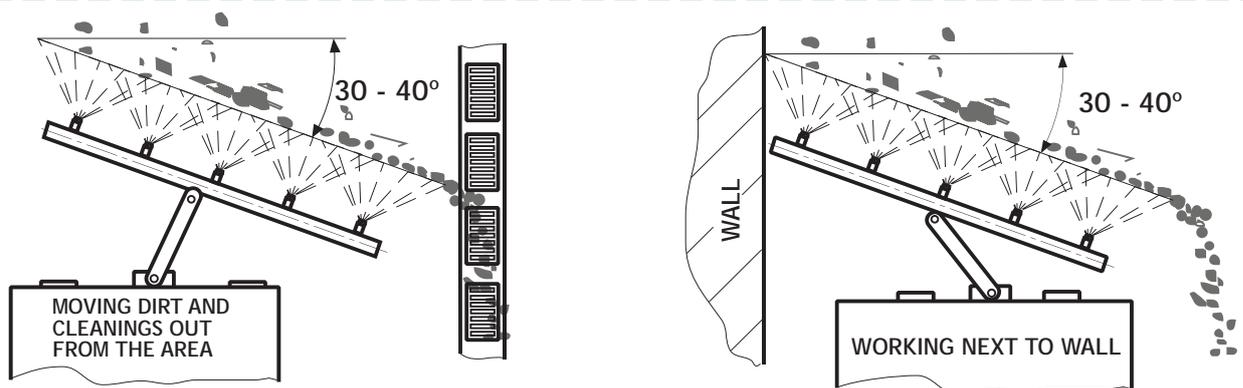
The steering angle of street washing pipe is determined by direction, where the dirt is being moved to. The angle of 30–40° is proved to be most effective - refer to the above sketches. High pressure water jets work as dozer blade, moving dirt and cleanings along the street washing pipe to its other end and further aside.
